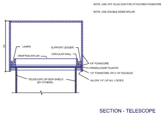
**Figure 1:** Example schematic of a lightbox (<http://www.gregpyros.com/assets/Lightbox-pyros.pdf>)
